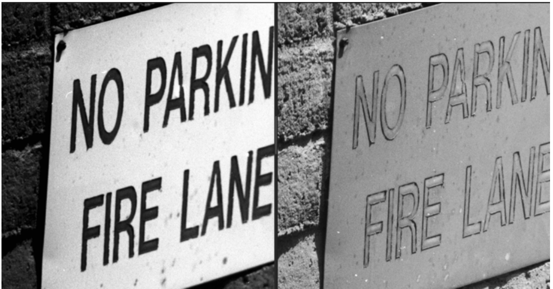
Infrared test, no focus adjustment between the initial focus and adding the IR 720nm filter:
